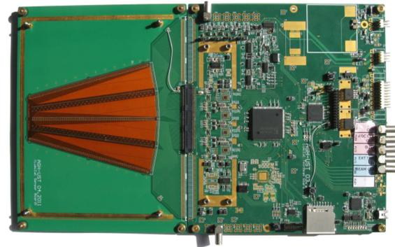
Figure 4. Prototype module of LumiCal detector
