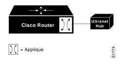
Data being transmitted from the router is returned to the router, and incoming data from outside is transmitted back outside.
