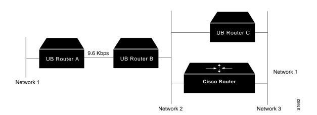
*Figure 1-1* Sample Ungermann-Bass Routing Configuration
