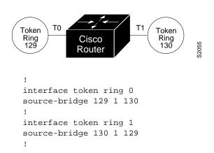
Token Rings 129 and 130 are connected via the Cisco router/bridge.
